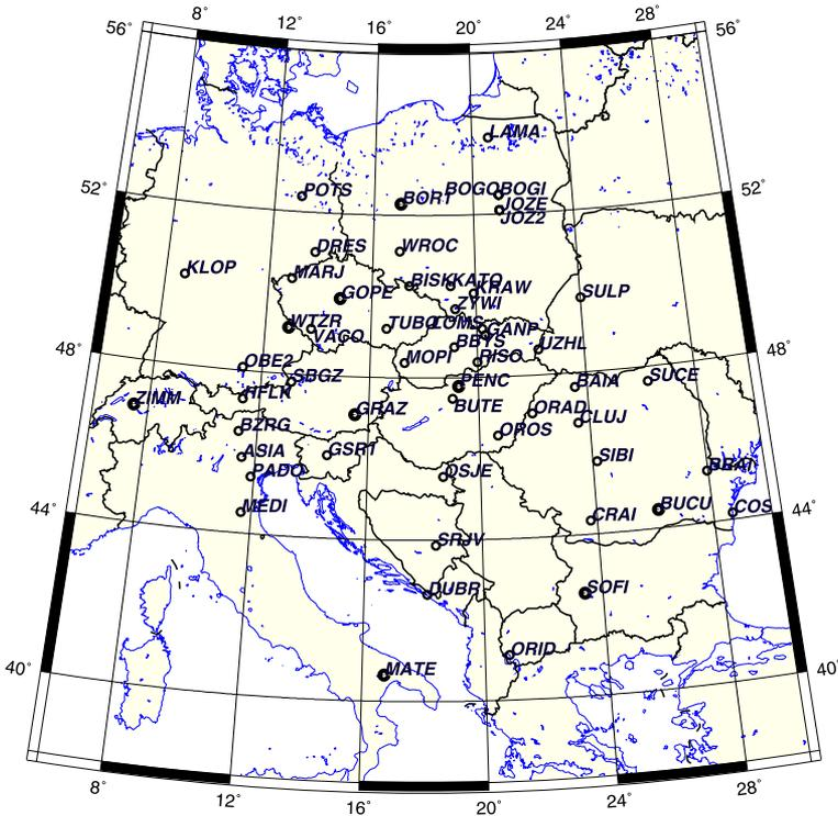
Fig. 1. Network of GNSS stations analyzed. Sites which are used for referencing to ITRF2005 are highlighted with full circles.
