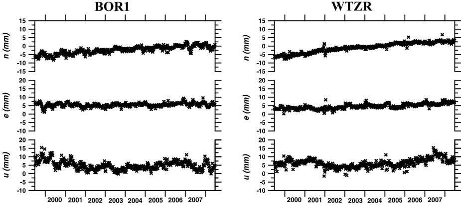
Fig. 5. Examples of stations where the linear change is dominated by the relatively slight coordinate variability.
