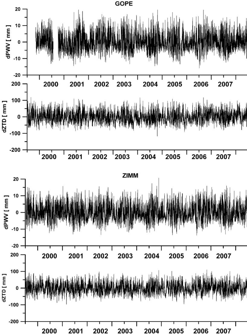
Fig. 10. Residual ZTD and PWV variations for stations GOPE and ZIMM after elimination of seasonal and diurnal periodic terms.
