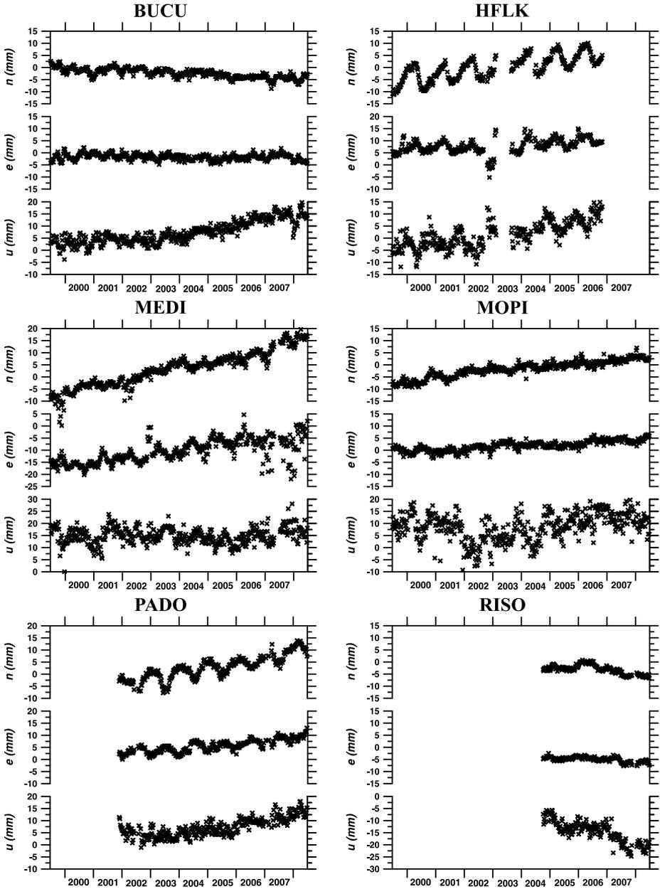
Fig. 6. Examples of stations where one or more coordinate components have a specific behavior.
