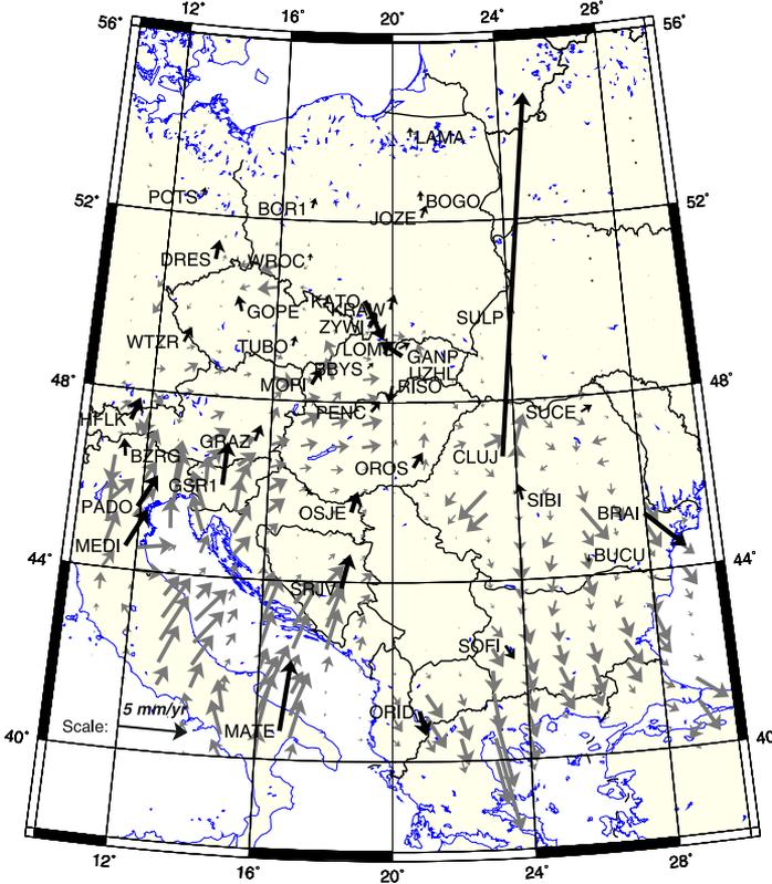
Fig. 7. Comparison of intraplate velocities obtained from the analysis in this paper (black vectors) with the interpolated velocity field (gray vectors) generated on the basis of various GNSS data in Hefty (2007).
