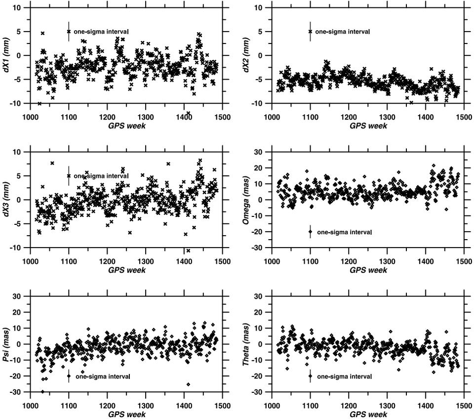
Fig. 4. Time series of transformation parameters estimated for linking the weekly coordinate solutions to ITRF2005. The one-sigma intervals show the mean values reflecting the consistency of estimated coordinates with ITRF2005 at identical points.
