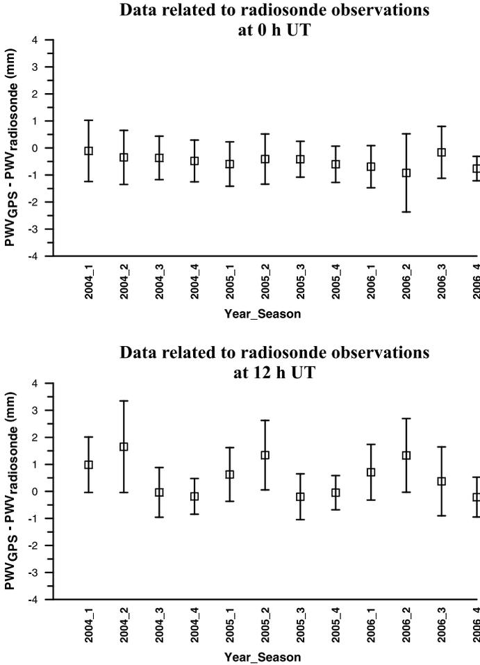
Fig. 11. Mean difference between PWV derived from GPS observations at GANP stations and PWV obtained from radiosonde measurements at Gánovce meteorological observatory.
