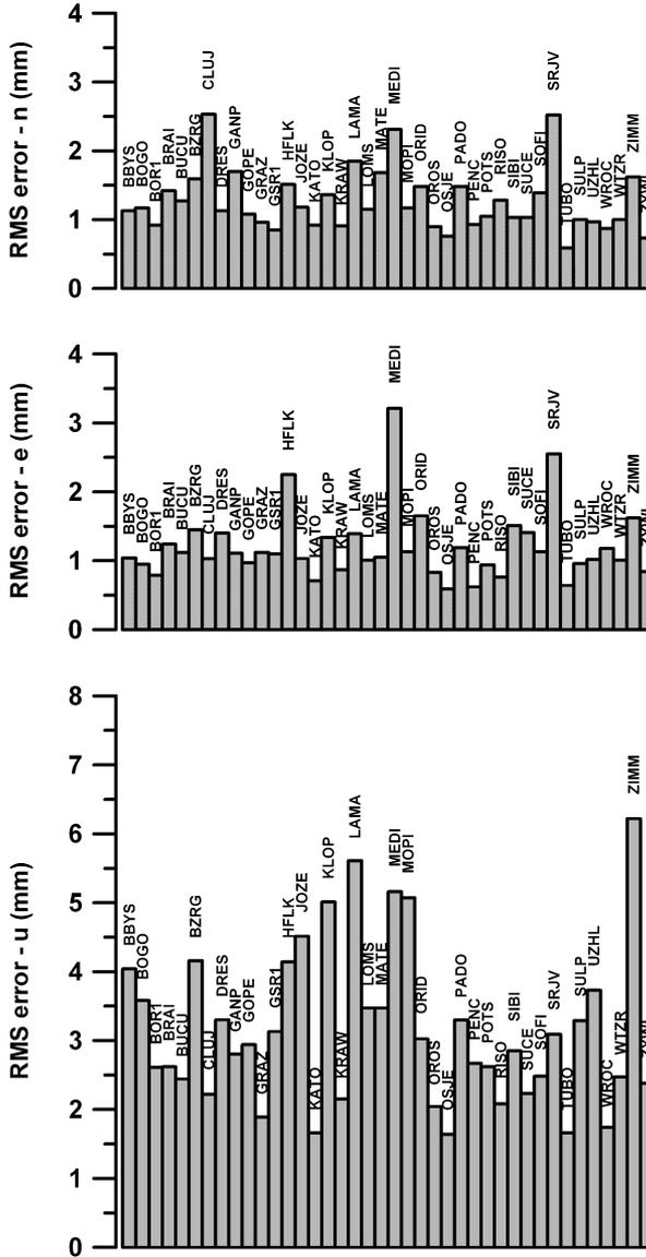
Fig. 8. Post-fit RMS errors of  $n$ ,  $e$  and  $u$  coordinate components of weekly solutions for sites exceeding 3-year interval of observations.
