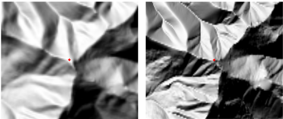
Fig. 9. Comparison of the DEM used in the older version CBA2G_SK 2015 (left) and the new version 2025 (right) in the area of the Kľak summit in Malá Fatra Mts. The red cross indicates the gravimetric point.
