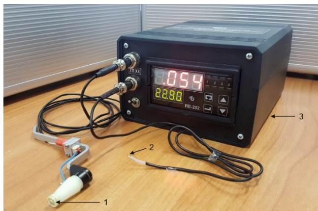
Fig.1. The appearance of the thermoelectric device for ophthalmology. 1 - thermoelectric heat flux sensor, 2 - thermocouple sensor, 3 - data acquisition unit.
