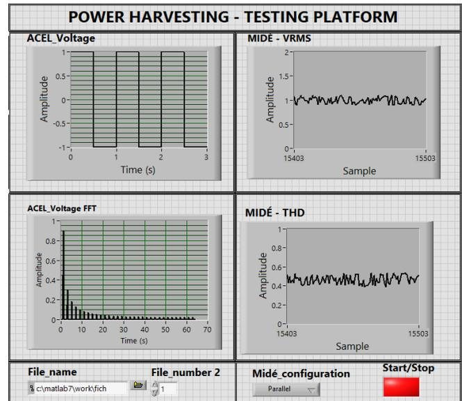
Fig.4. Front panel of the LabVIEW program used to display results of the acceleration data (left side) and power harvesting device (right side).
