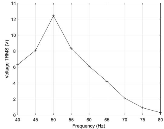
Fig.6. Frequency response of the power harvesting module tuned for a natural frequency of 50 Hz.
