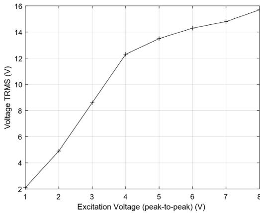
Fig.8. RMS voltage delivered by the piezoelectric module for a sinusoidal exciting voltage with a frequency equal to 50 Hz with amplitude values varying between 1 and 8 V with increments of 1 V.
