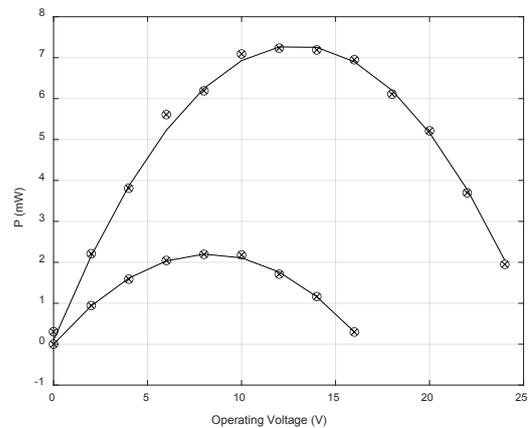
Fig.9. Experimental results of the harvested power as a function of the operating voltage (upper curve- 1 g acceleration; lower curve- 0.5 g acceleration; dotted points- experimental values; continuous line- polynomial curve fitted values).
