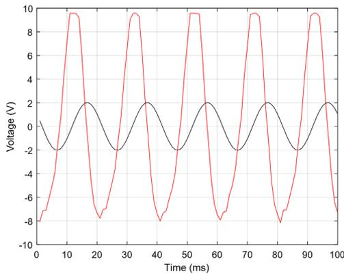
Fig.5. Experimental results obtained for a sinusoidal voltage with null offset, 2 V amplitude and 50 Hz frequency applied to the vibration exciter (black curve) and the open-circuit output voltage delivered by the power harvesting module (red curve).
