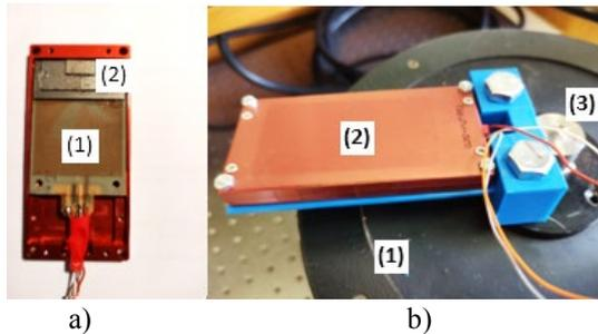
Fig.3. Piezoelectric module and vibration exciter used for testing purposes: a) Detailed view of the piezoelectric module and dimensional scale reference: (1) piezoelectric wafers; (2) tuning tip mass; (3) 1 € coin relative dimensional scale; b) Assembly details of the interconnection between the vibration exciter and the piezoelectric module: (1) vibration exciter; (2) piezoelectric module; (3) vibration exciter accelerometer.
