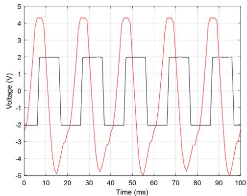
Fig.7. Time response of the power harvesting module for a square waveform excited vibration with a null offset and an amplitude equal to 2 V.
