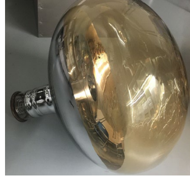
Fig.2. The 20-inch coated MCP-PMT sample developed in XIOPM.
