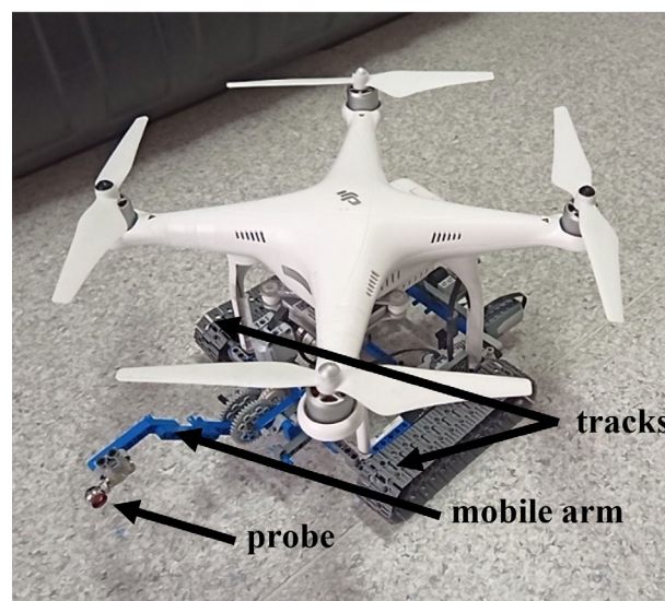
Fig.1. DJI Phantom 3 drone with the prototype landing gear and the mobile arm with the probe.
