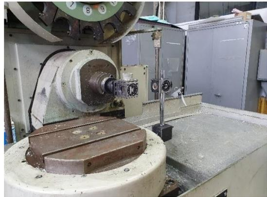
Fig. 7. Interferometer and reflector on the work table.
