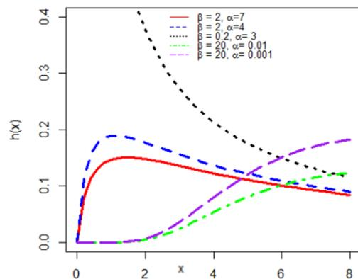
Fig. 2. The shape of the failure rate function of the  $\alpha$ PIP distribution.
