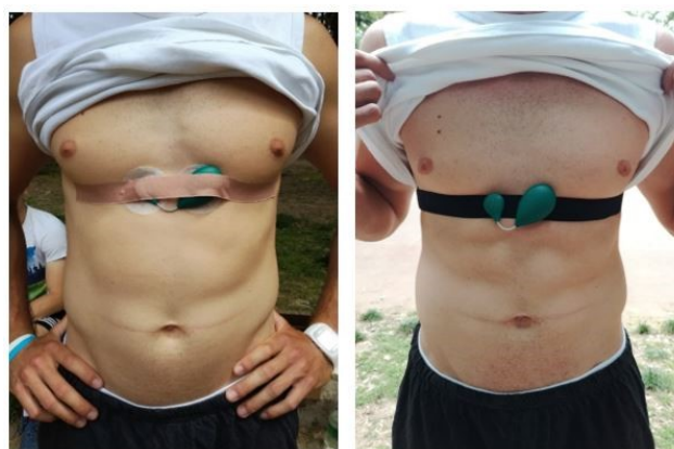
Fig.1. LI position of the sensor and electrodes fixed with tape in the first test (left) and in the second test (right), where sensor was fixed with Polar soft-strap belt.
