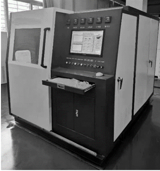
Fig.1. Hydraulic pump test platform.
