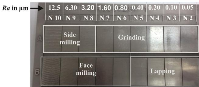
Fig. 1. Rugotest used in the experiment.
