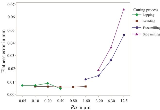
Fig.5. The effect of the cutting process and quality of the machined surface on flatness error.
