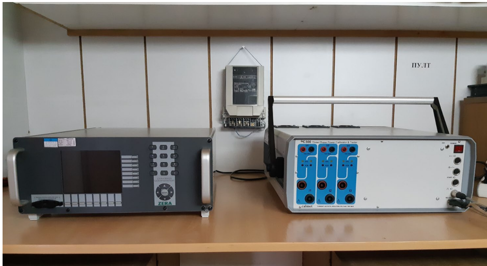
Fig.1. Primary and secondary reference standards of LEM in the domain of electrical power and energy.
