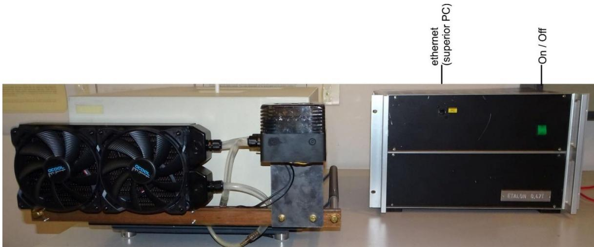
Fig. 4. Benchmark from the front. The NMR sample cooling device is mounted on a permanent magnet housing.
