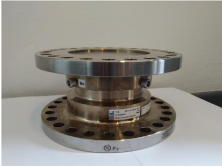
Fig. 1. The HBK special torque transducer with a lifting capacity of 2000 N·m and a sensitivity of 1.0 mV/V designed to measure clockwise and anti-clockwise torque.
