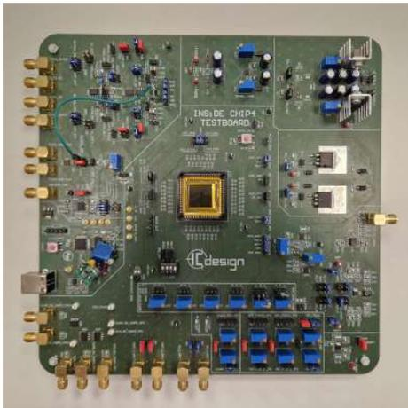
Fig. 8. Developed test board for the evaluation of FDDA samples.
