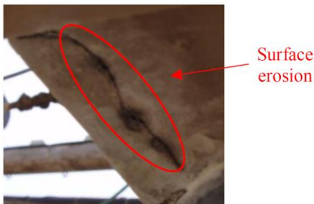
Fig. 4. The effect of boundary surface electrical strength in the aging test process of HV electrical apparatus insulation material.
