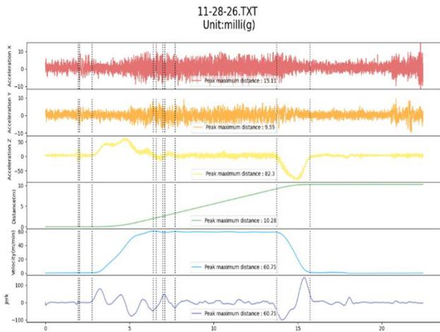
Fig. 17. Abnormal elevator operation with eleven segments.
