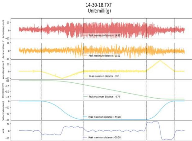
Fig. 13. Normal elevator operation within three floors.
