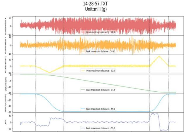
Fig. 14. Normal elevator operation within four floors.
