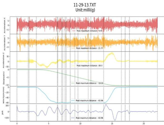
Fig. 18. Abnormal elevator operation with twenty-one segments.
