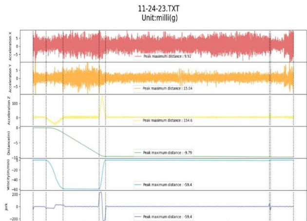
Fig. 16. Abnormal elevator operation with nine segments.
