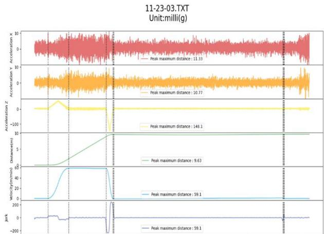
Fig. 15. Abnormal elevator operation with six segments.
