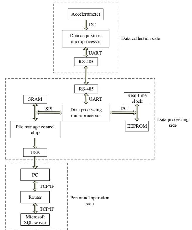
Fig. 1. System structure.
