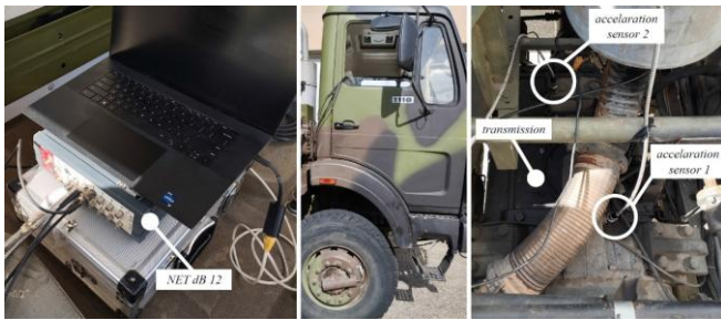
Fig. 4. Measurement device and vehicle FAP 1118, 4x4.
