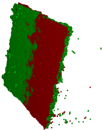
Fig. 5. Pose is calculated using the CPD algorithm and the point clouds were aligned based on estimates leading to errors.
