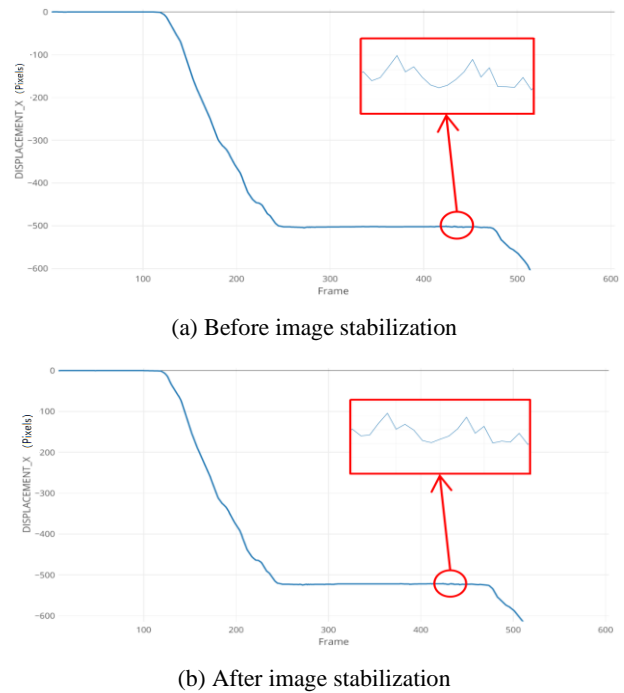
Fig. 2. Comparison of the displacement curve between before and after image stabilization at 30 m.
