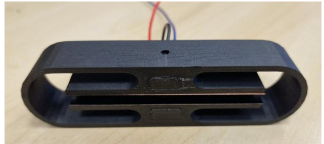
Fig. 9. Manufactured sensor of mechanical quantity from the PET-G body.
